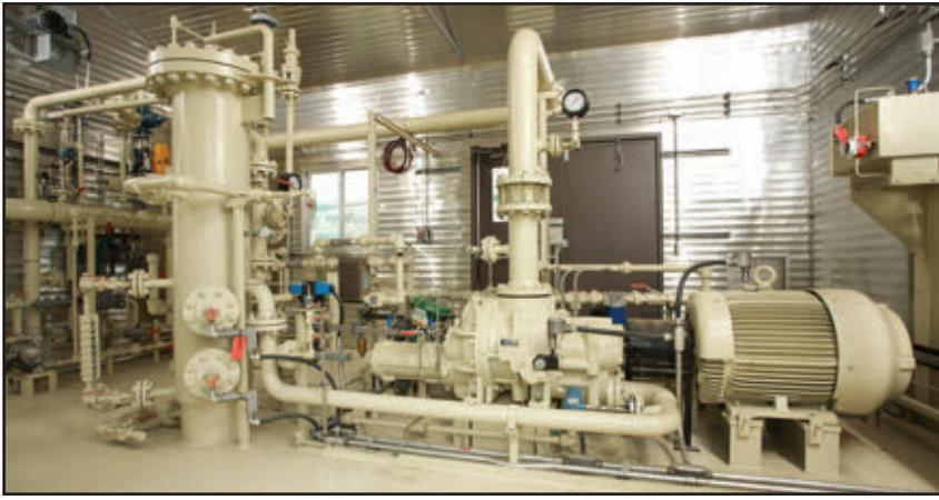
**All of the packages are skid-mounted and come with insulated buildings and heaters for cold weather operation.**
