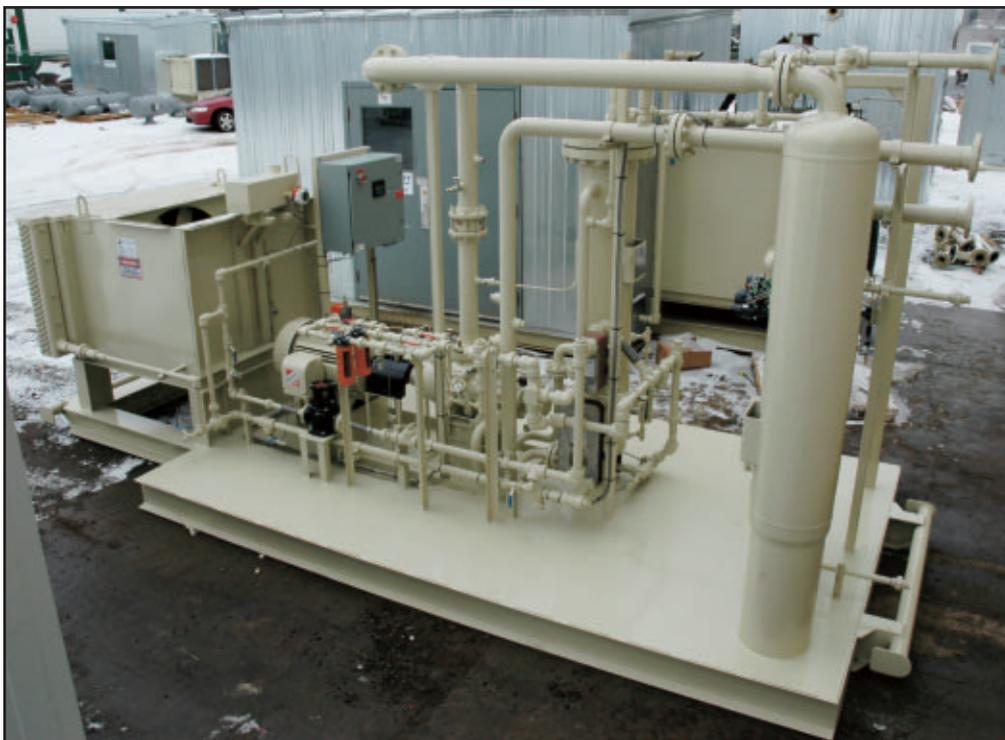
The packages range from 50 to 350 hp (37 to 260 kW), using Sullair or Frick screw compressors, depending on the required pressure.
